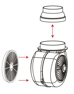
Reducer Collar reduces the motor exhaust from 150mm to 125mm if required (Already supplied in box)
